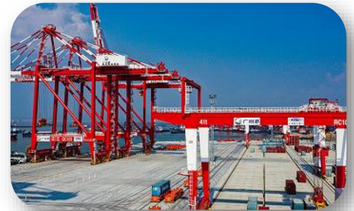
Large-scale deployment of automated single trolley quay cranes
