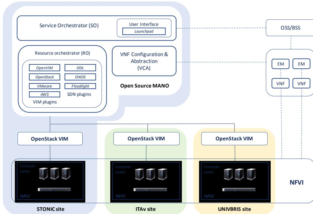
**Figure 2: Architectural design of the 5GinFIRE MANO platform**
