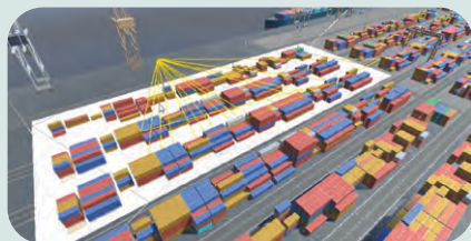
Figure 4. 5G coverage study in a container terminal with the Fivecomm planning tool.
