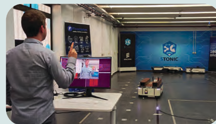
Figure 5. Fivecomm software platform used in the context of 5G-INDUCE for remote control of AGVs.
