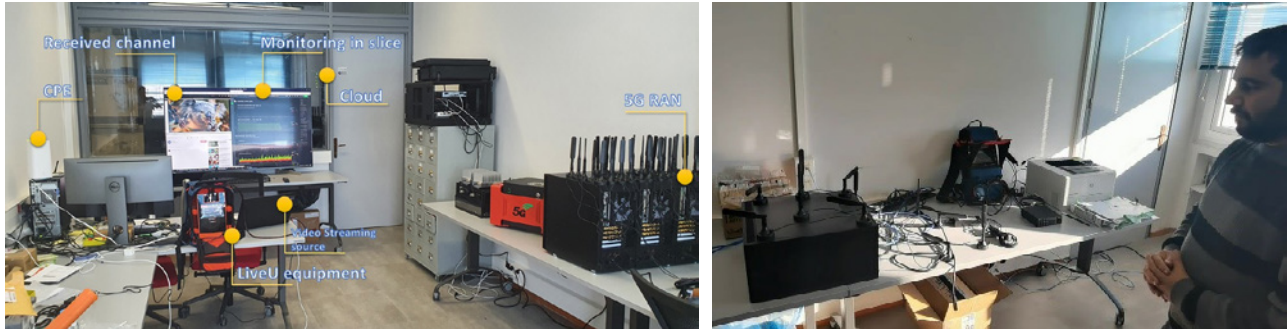
Figure 2: LiveU Deployment Setup and LiveU unit and 5G base station at University of Patras
