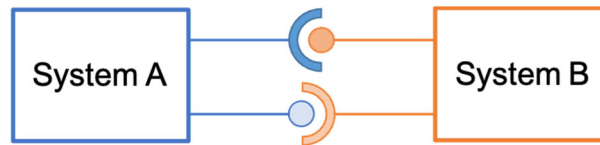
Figure 2-3: Mutually providing and accessing services between systems
