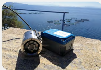
Camera to be installed underwater, for monitoring the production, and to transmit through cabling and 4G/5G and fault management
