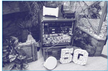
Fig. 36: 5G private network Core and baseband unit
