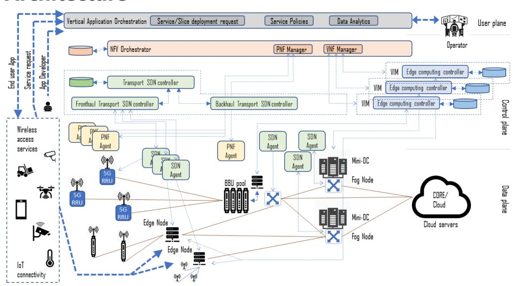
A fully operational **5G system platform** from the user end to the data plane
