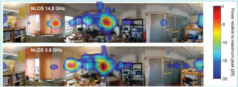
Figure 18: Directional power distribution in an office environment
