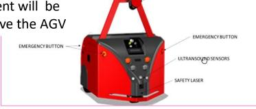
Simultaneous localization and mapping (SLAM) Navigation Safety Laser Radio Wi-Fi
