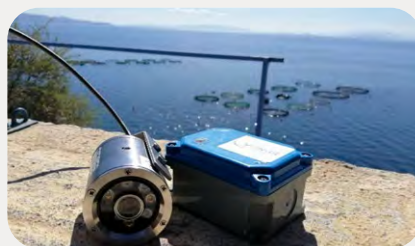
Figure 2: Camera to be installed underwater, for monitoring the production, and to transmit through cabling and 4G/5G.
