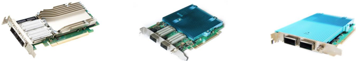
Figure 11. Netcope platform (left: NFB-200G2QL; middle: NFB-100G2Q; right: NFB-100G2C) [24]
